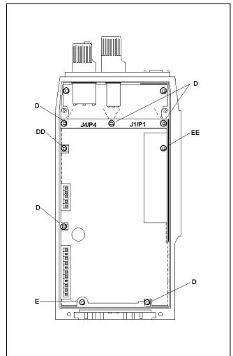
Figure 8 - Control Board Access
